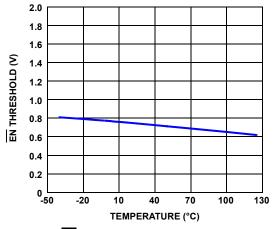
FIGURE 20. EN INPUT THRESHOLD vs TEMPERATURE
