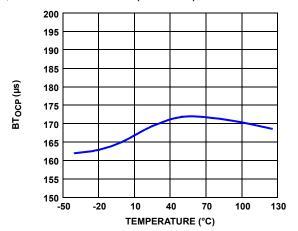
FIGURE 15. OVERCURRENT PROTECTION BLANKING TIME vs TEMPERATURE
