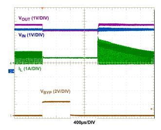
FIGURE 13. BYPASS FUNCTIONALITY ( $V_{IN} = 3V$ ,  $V_{OUT} = 3.3$ , 0.5A R<sub>LOAD</sub>)
