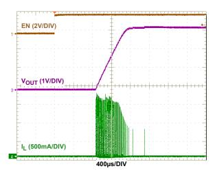
FIGURE 6. SOFT-START ( $V_{IN} = 4V$ ,  $V_{OUT} = 3.3V$ , NO LOAD)
