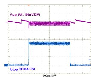
FIGURE 10. OA TO 0.5A LOAD TRANSIENT ( $V_{IN} = 4V$ ,  $V_{OUT} = 3.3V$ )
