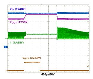
FIGURE 12. BYPASS FUNCTIONALITY ( $V_{IN} = 4V$ ,  $V_{OUT} = 3.3$ , 0.5A R<sub>LOAD</sub>)
