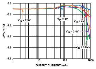
FIGURE 4. OUTPUT VOLTAGE vs OUTPUT CURRENT
