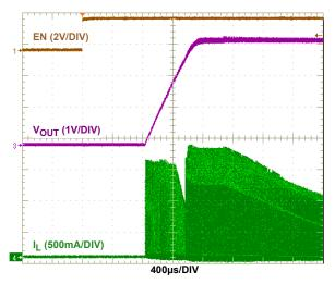
FIGURE 9. SOFT-START ( $V_{IN} = 3V$ ,  $V_{OUT} = 3.3V$ , 0.5A  $R_{LOAD}$ )
