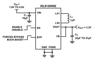
FIGURE 1. TYPICAL FIXED OUTPUT APPLICATION
