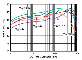
FIGURE 2. EFFICIENCY: V<sub>OUT</sub> = 3.3V, T<sub>A</sub> = +25°C
