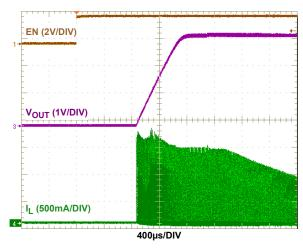
FIGURE 7. SOFT-START ( $V_{IN}$  = 4V,  $V_{OUT}$  = 3.3V, 0.5A  $R_{LOAD}$ )
