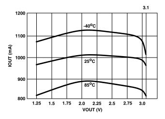
FIGURE 4. CURRENT REGULATION vs VOUT (VIN = 3.3V)
