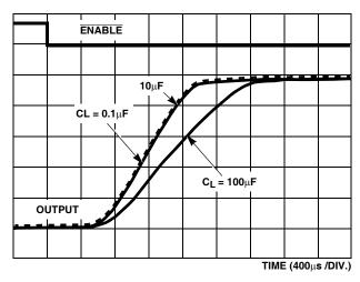
FIGURE 3. VOUT SOFT START vs  $\text{C}_{\text{LOAD}},\,\text{RI}$  =10 $\!\Omega$
