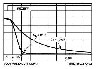
FIGURE 8. SLOW TURN -OFF vs C\_LOAD, RI = 10 $\!\Omega$
