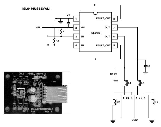
FIGURE 20. ISL6436USBEVAL BOARD
