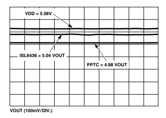
FIGURE 13. ISL6436 vs PPTC INTO 500mA LOAD
