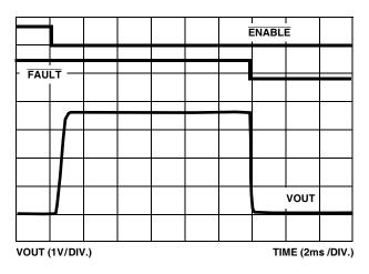
FIGURE 10. ISL6436L TURN-ON INTO 1.5A OCS
