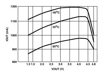
FIGURE 5. CURRENT REGULATION vs VOUT (VIN = 5.0V)
