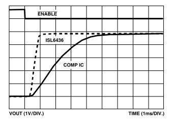
FIGURE 16. COMPARATIVE TURN-ON WAVEFORMS, RI =  $10\Omega$
