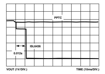
FIGURE 14. ISL6436 vs PPTC PLUGGED ONTO 1.5A LOAD
