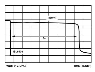
FIGURE 15. ISL6436 vs PPTC WITH EXTENDED 1.5A LOAD
