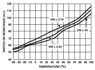
FIGURE 2. SWITCH ON RESISTANCE AT 0.7A
