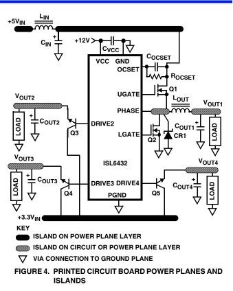
The critical small signal components include the bypass capacitor for VCC and the feedback resistors. Locate these components close to their connecting pins on the control IC.
