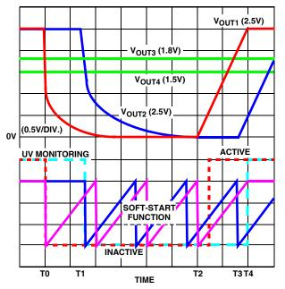
FIGURE 1. OVERCURRENT/UNDERVOLTAGE PROTECTION RESPONSE
