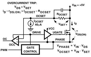
FIGURE 2. OVERCURRENT DETECTION
