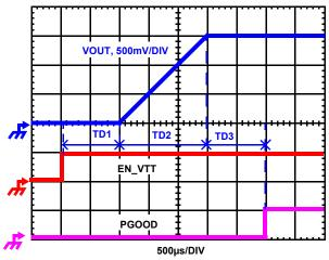
FIGURE 11. SOFT-START WAVEFORMS
