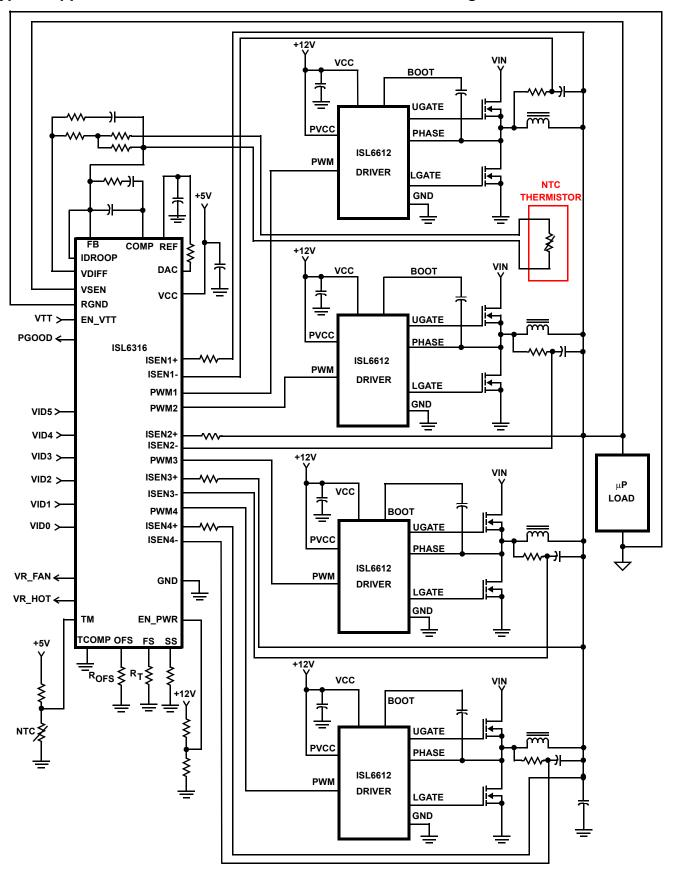
Typical Application - 4-Phase Buck Converter with DCR Sensing and Integrated TCOMP
