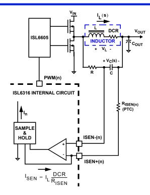
FIGURE 4. DCR SENSING CONFIGURATION
