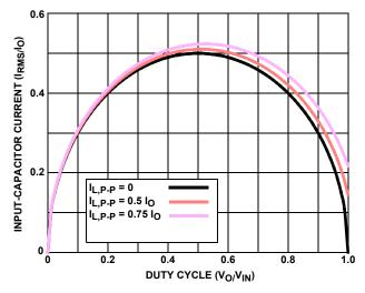
FIGURE 24. NORMALIZED INPUT-CAPACITOR RMS
