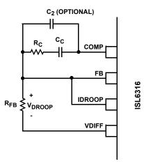
FIGURE 19. COMPENSATION CONFIGURATION FOR LOAD-LINE REGULATED ISL6316 CIRCUIT
