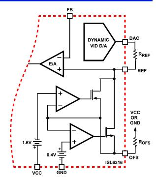
FIGURE 9. OUTPUT VOLTAGE OFFSET PROGRAMMING
