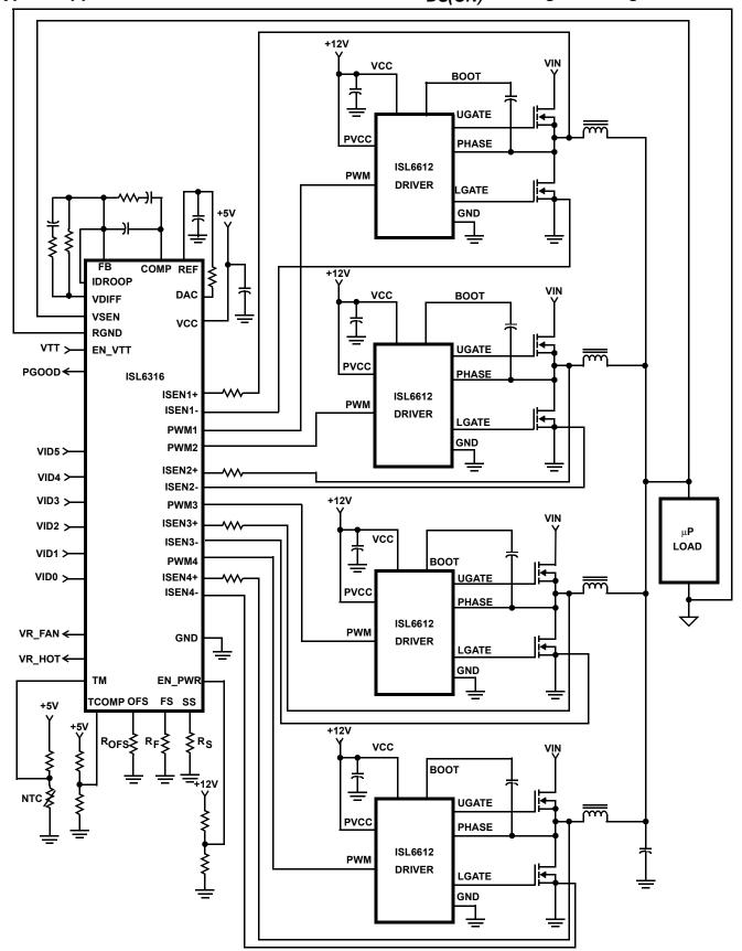
Typical Application - 4-Phase Buck Converter with DCR Sensing and External TCOMP
