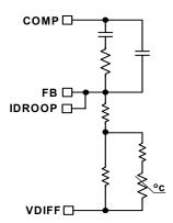
FIGURE 18. VOLTAGE AT IDROOP PIN WITH A RESISTOR
