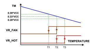
FIGURE 16. VR\_HOT AND VR\_FAN SIGNAL vs TM VOLTAGE
