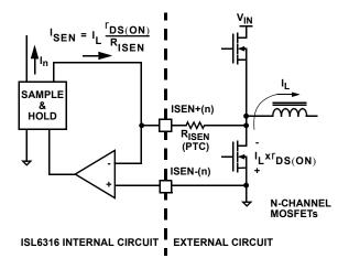
FIGURE 6. MOSFET r<sub>DS(ON)</sub> CURRENT-SENSING CIRCUIT
