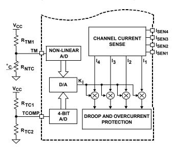
FIGURE 17. BLOCK DIAGRAM OF INTEGRATED TEMPERATURE COMPENSATION
