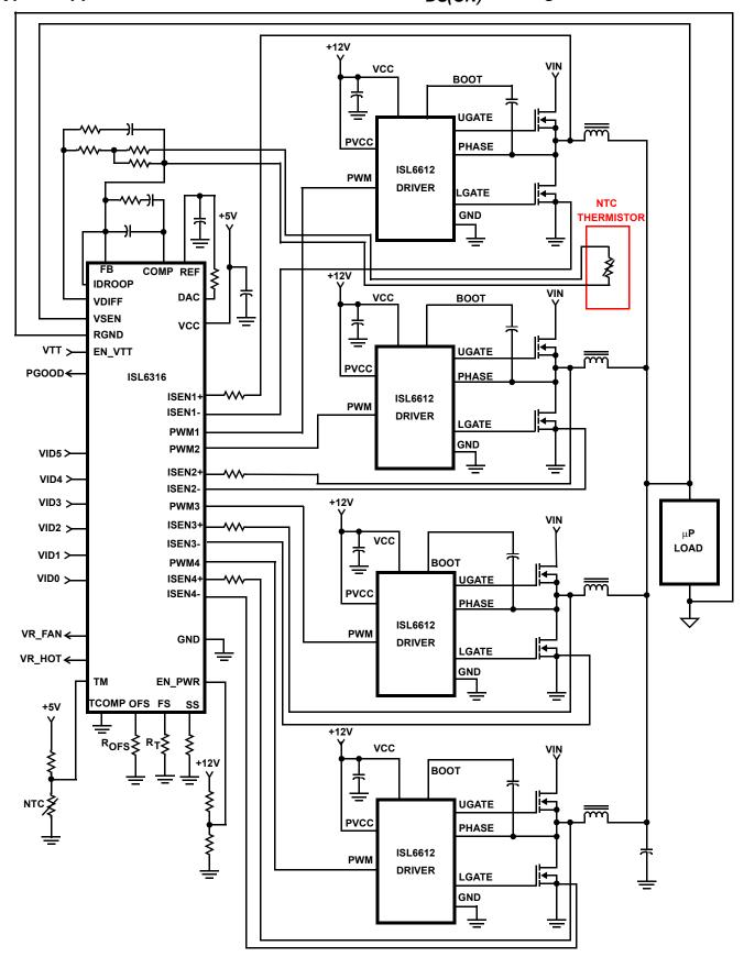
Typical Application - 4-Phase Buck Converter with r<sub>DS(ON)</sub> Sensing and Integrated TCOMP
