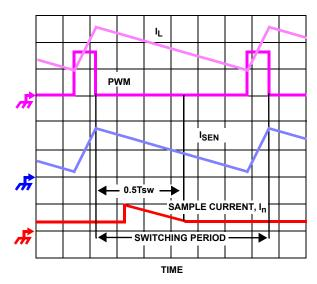
FIGURE 3. SAMPLE AND HOLD TIMING
