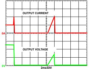
FIGURE 13. OVERCURRENT BEHAVIOR IN HICCUP MODE.  $F_{SW} = 500 \text{kHz}$
