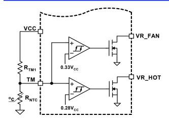
FIGURE 14. BLOCK DIAGRAM OF THERMAL MONITORING FUNCTION
