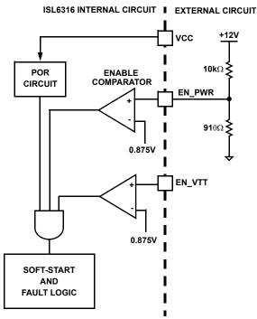
FIGURE 10. POWER SEQUENCING USING THRESHOLD-SENSITIVE ENABLE (EN) FUNCTION
