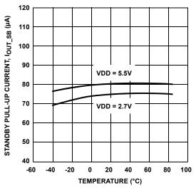
FIGURE 3. STANDBY PULL-UP CURRENT, DDC1,  $2 = V_{DD} - 0.5V$
