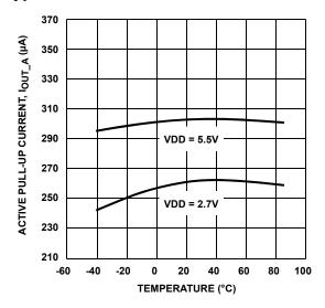
FIGURE 1. ACTIVE PULL-UP CURRENT, DDC PIN = 0V
