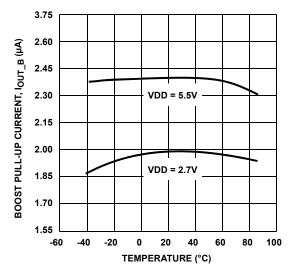
FIGURE 2. BOOST PULL-UP CURRENT, DDC PIN =  $V_{DD}/2$
