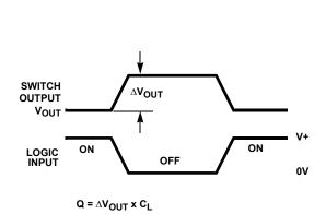
FIGURE 2A. MEASUREMENT POINTS
