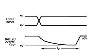
FIGURE 3A. MEASUREMENT POINTS
