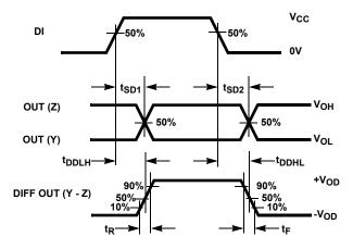
$t_{SSK} = |t_{SD1(Y)} - t_{SD2(Y)}| \text{ OR } |t_{SD1(Z)} - t_{SD2(Z)}| \qquad t_{DSK} = |t_{DDLH} - t_{DDHL}|$
