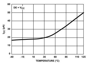
FIGURE 8. STATIC SUPPLY CURRENT vs TEMPERATURE
