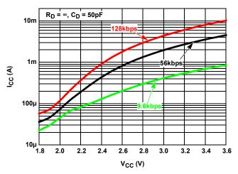
FIGURE 9. ISL32613E DYNAMIC SUPPLY CURRENT vs SUPPLY VOLTAGE AT DIFFERENT DATA RATES
