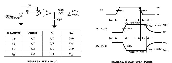
FIGURE 6. DRIVER ENABLE AND DISABLE TIMES
