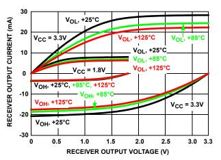
FIGURE 25. ISL32602E, ISL32603E RECEIVER OUTPUT CURRENT vs RECEIVER OUTPUT VOLTAGE
