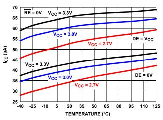
FIGURE 12. ISL32600E, ISL32601E STATIC SUPPLY CURRENT vs TEMPERATURE
