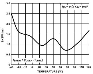
FIGURE 17. ISL32600E, ISL32601E DRIVER DIFFERENTIAL SKEW vs TEMPERATURE
