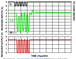
FIGURE 29. ISL32602E, ISL32603E PERFORMANCE WITH V<sub>CC</sub> = 3.3V, 460kbps, 2000ft (610m) CAT 5 CABLE
