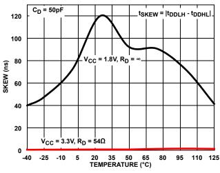
FIGURE 31. ISL32602E, ISL32603E DRIVER DIFFERENTIAL SKEW vs TEMPERATURE
