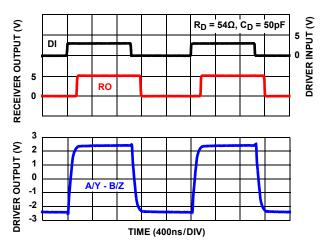
FIGURE 24.  $V_{CC}$  = 5V, DRIVER AND RECEIVER WAVEFORMS (ISL32433E, ISL32435E)
