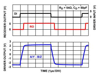
FIGURE 23. V<sub>CC</sub> = 5V, DRIVER AND RECEIVER WAVEFORMS (ISL32430E, ISL32432E, ISL32437E)
