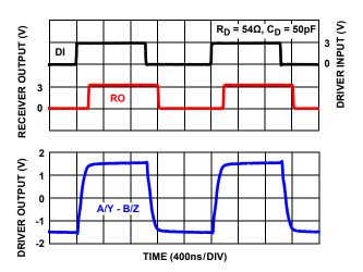
FIGURE 22.  $V_{CC}$  = 3.3V, DRIVER AND RECEIVER WAVEFORMS (ISL32433E, ISL32435E)
