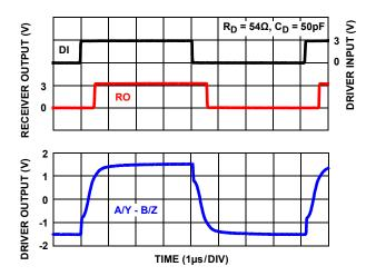
FIGURE 21.  $V_{CC}$  = 3.3V, DRIVER AND RECEIVER WAVEFORMS (ISL32430E, ISL32437E)
