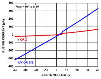
FIGURE 13. BUS PIN CURRENT vs BUS PIN VOLTAGE
