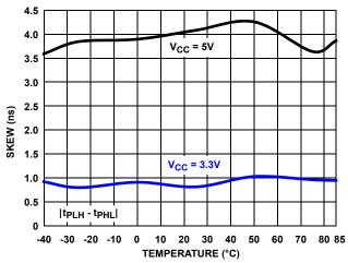
FIGURE 18. DRIVER DIFFERENTIAL SKEW vs TEMPERATURE (ISL32433E, ISL32435E)
