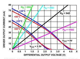
FIGURE 9. DRIVER OUTPUT CURRENT vs DIFFERENTIAL OUTPUT VOLTAGE
