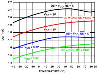
FIGURE 11. SUPPLY CURRENT vs TEMPERATURE
