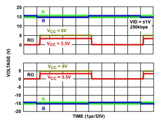
FIGURE 19. ±15V RECEIVER PERFORMANCE (ISL32430E, ISL32432E, ISL32437E)
