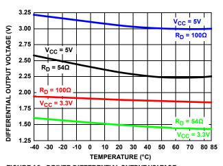
FIGURE 10. DRIVER DIFFERENTIAL OUTPUT VOLTAGE VS TEMPERATURE
