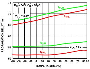
FIGURE 17. DRIVER DIFFERENTIAL PROPAGATION DELAY vs TEMPERATURE (ISL32433E, ISL32435E)
