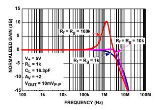
FIGURE 1. GAIN vs FREQUENCY vs FEEDBACK RESISTOR VALUES  $R_f/R_\alpha$
