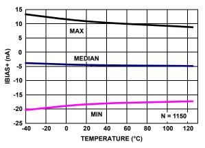
FIGURE 26. IBIAS+ vs TEMPERATURE, V+, V\_ = ±1.2V
