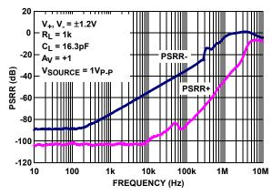
FIGURE 10. PSRR vs FREQUENCY, V<sub>+</sub>, V<sub>-</sub> = ±1.2V
