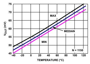
FIGURE 35.  $V_{OUT}$  LOW vs TEMPERATURE  $V_+$ ,  $V_- = \pm 2.5V$ ,  $R_1 = 1k$
