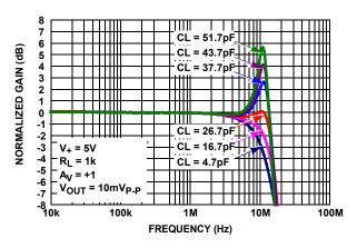
FIGURE 8. GAIN vs FREQUENCY vs CL
