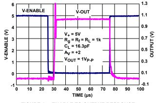
FIGURE 17. ENABLE TO OUTPUT RESPONSE
