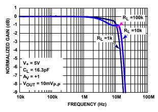
FIGURE 5. GAIN vs FREQUENCY vs RL
