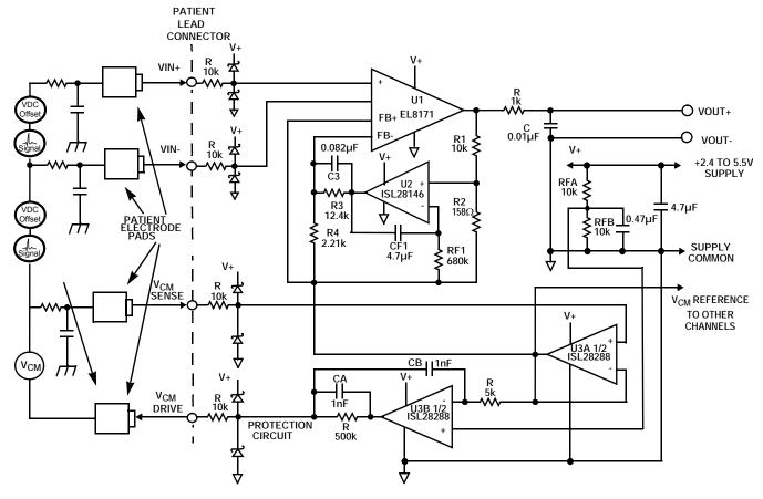
FIGURE 38. ECG/EEG AMPLIFIER
