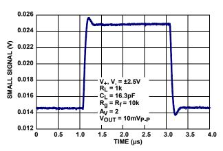
FIGURE 16. SMALL SIGNAL STEP RESPONSE
