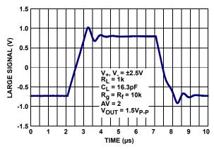
FIGURE 15. LARGE SIGNAL STEP RESPONSE
