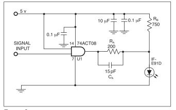
FIGURE 3. Test application circuit (IF = 22mA).
