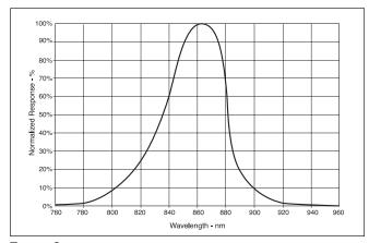
FIGURE 2. Typical spectral output vs. wavelength.
