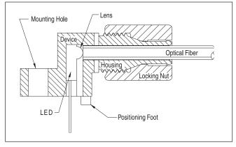
FIGURE 4. Cross-section of fiber optic device.
