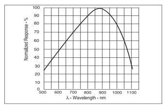
$Figure \ 1.$  Typical detector response versus wavelength.
