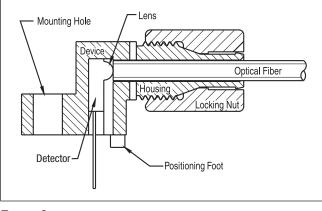
Figure 3. Cross-section of fiber optic device.
