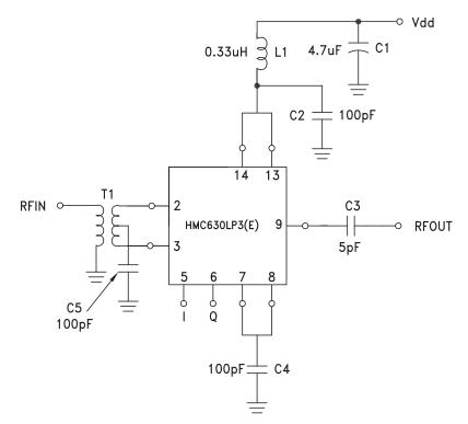
\* Pins 15 & 16 are redundant I & Q inputs.
