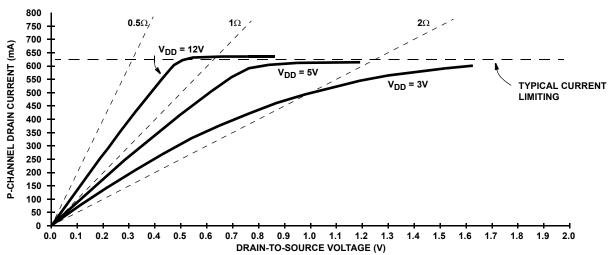
FIGURE 5. TYPICAL CHARACTERISTIC OF THE P-MOSFET OUTPUT DRIVER DRAIN CURRENT vs DRAIN-TO-SOURCE VOLTAGE,
