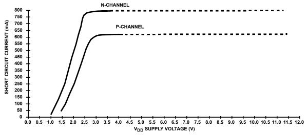
FIGURE 7. TYPICAL CHARACTERISTIC OF THE P AND N OUTPUT DRIVER SHORT CIRCUIT CURRENT vs SUPPLY VOLTAGE,
