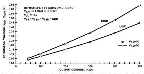
FIGURE 8. TYPICAL CHARACTERISTIC OF SATURATION VOLTAGE vs OUTPUT CURRENT USING A +5V SUPPLY, TAMBIENT = 25°C
