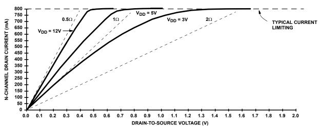
FIGURE 6. TYPICAL CHARACTERISTIC OF THE N-MOSFET OUTPUT DRIVER DRAIN CURRENT vs DRAIN-TO-SOURCE VOLTAGE,  $T_{AMBIENT} = 25^{\circ}C$
