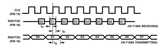
FIGURE 2A. SERIAL MODE 0 TIMING
