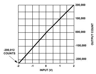
FIGURE 9. TYPICAL HI-7159A TRANSFER CHARACTERISTIC
