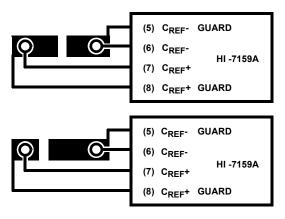
FIGURE 10. TYPICAL GUARD RING LAYOUT
