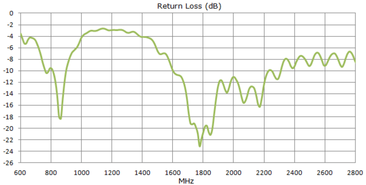
Figure 3. Return Loss of G30 Antenna on 30x30cm metal
