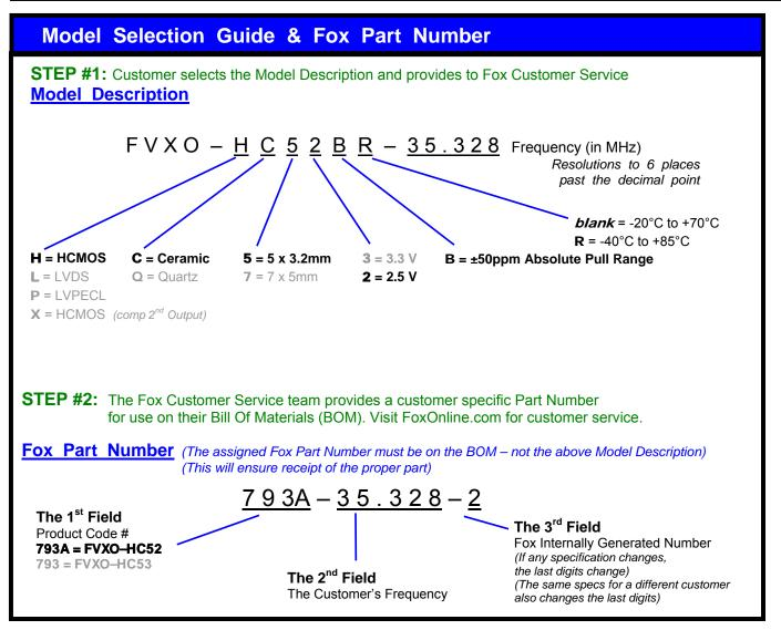
This example, FVXO-HC52BR-35.328 = Voltage Controlled, HCMOS Output, Ceramic, 5 x 3.2mm Package, 2.5V, ±50 PPM Absolute Pull Range, -40 to +85°C Temperature Range, at 35.328 MHz
