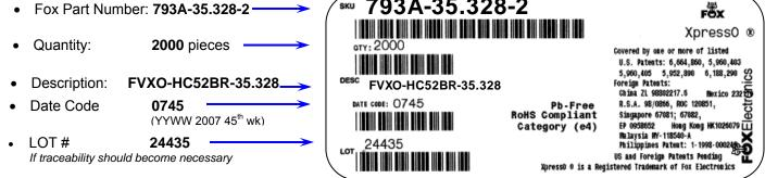
An additional identification code is contained internally if tracking should ever be necessary
