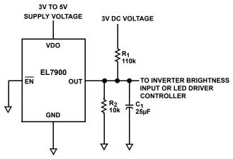
FIGURE 10. AUTOMATIC DIMMING SOLUTION
