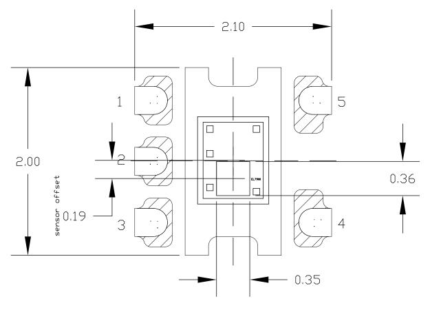
FIGURE 13. EL7900 SENSOR DIAGRAM
