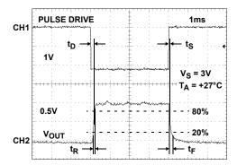
FIGURE 2. RISE/FALL TIME MEASUREMENT WAVEFORMS
