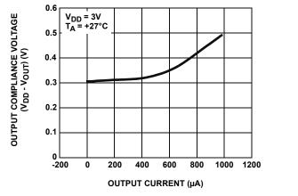
FIGURE 7. OUTPUT COMPLIANCE VOLTAGE vs CURRENT
