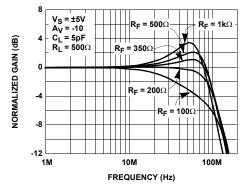
FIGURE 3. INVERTING FREQUENCY RESPONSE FOR VARIOUS RF
