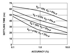
FIGURE 27. SETTLING TIME vs ACCURACY
