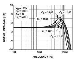
FIGURE 14. NON-INVERTING FREQUENCY RESPONSE FOR VARIOUS CL
