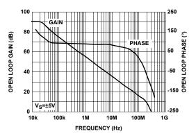
FIGURE 17. OPEN LOOP GAIN AND OPEN LOOP PHASE
