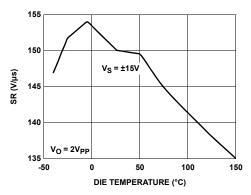
FIGURE 43. SLEW RATE vs TEMPERATURE
