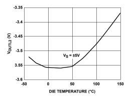
FIGURE 46. NEGATIVE LOADED OUTPUT SWING vs **TEMPERATURE**
