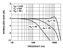
FIGURE 8. INVERTING FREQUENCY RESPONSE FOR VARIOUS RF
