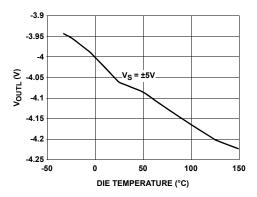
FIGURE 40. NEGATIVE OUTPUT SWING vs TEMPERATURE
