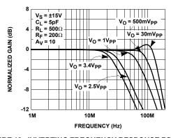
FIGURE 12. INVERTING FREQUENCY RESPONSE FOR VARIOUS OUTPUT SIGNAL LEVELS
