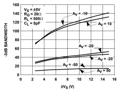
FIGURE 19. BANDWIDTH vs Vs
