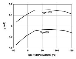
FIGURE 34. SUPPLY CURRENT vs TEMPERATURE
