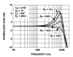
FIGURE 2. NON-INVERTING FREQUENCY RESPONSE FOR VARIOUS RF
