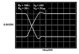
FIGURE 21. LARGE SIGNAL STEP RESPONSE
