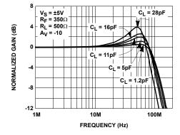
FIGURE 15. INVERTING FREQUENCY RESPONSE FOR VARIOUS CL
