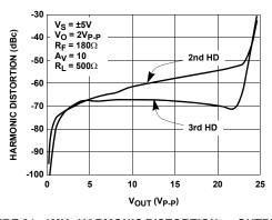
FIGURE 24. 1MHz HARMONIC DISTORTION vs OUTPUT SWING
