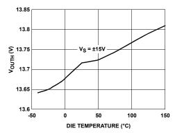
FIGURE 39. POSITIVE OUTPUT SWING vs TEMPERATURE
