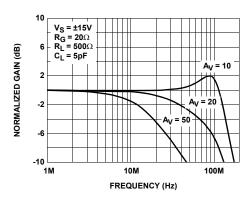
FIGURE 6. NON-INVERTING FREQUENCY RESPONSE FOR VARIOUS GAIN
