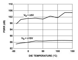
FIGURE 37. PSRR vs TEMPERATURE
