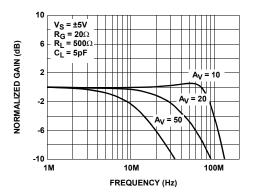
FIGURE 5. NON-INVERTING FREQUENCY RESPONSE FOR VARIOUS GAIN
