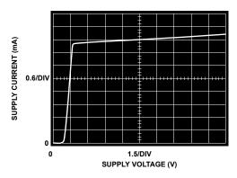
FIGURE 18. SUPPLY CURRENT vs SUPPLY VOLTAGE
