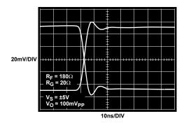
FIGURE 22. SMALL SIGNAL STEP RESPONSE
