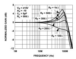
FIGURE 4. INVERTING FREQUENCY RESPONSE FOR VARIOUS RF
