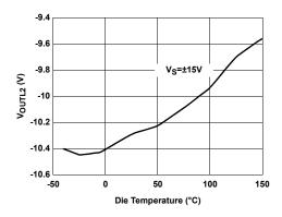
FIGURE 47. NEGATIVE LOADED OUTPUT SWING vs TEMPERATURE
