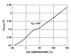
FIGURE 38. POSITIVE OUTPUT SWING vs TEMPERATURE
