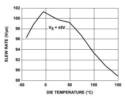
FIGURE 42. SLEW RATE vs TEMPERATURE
