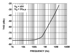
FIGURE 25. TOTAL HARMONIC DISTORTION vs FREQUENCY
