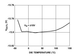
FIGURE 41. NEGATIVE OUTPUT SWING vs TEMPERATURE
