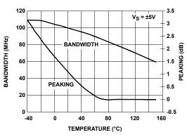
FIGURE 32. BANDWIDTH AND PEAKING vs TEMPERATURE
