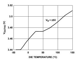
FIGURE 44. POSITIVE LOADED OUTPUT SWING vs **TEMPERATURE**
