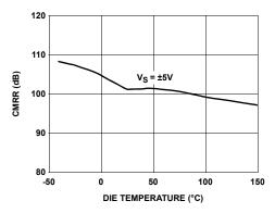
FIGURE 36. CMRR vs TEMPERATURE
