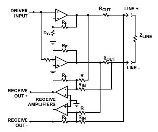
FIGURE 51. TYPICAL LINE INTERFACE CONNECTION
