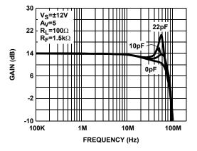
FIGURE 14. FREQUENCY RESPONSE vs C<sub>LOAD</sub> (EL1507CL - FULL POWER MODE)
