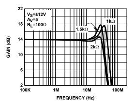
FIGURE 12. DIFFERENTIAL FREQUENCY RESPONSE vs R<sub>F</sub> (EL1507CL - 1/2 POWER MODE)
