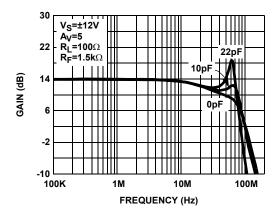
FIGURE 13. FREQUENCY RESPONSE vs C<sub>LOAD</sub> (EL1507CS - FULL POWER MODE)
