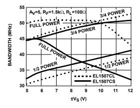
FIGURE 19. DIFFERENTIAL BANDWIDTH vs SUPPLY VOLTAGE
