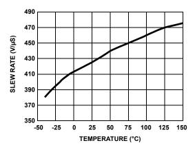
FIGURE 44. SLEW RATE vs TEMPERATURE
