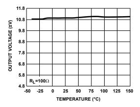
FIGURE 46. OUTPUT VOLTAGE vs TEMPERATURE
