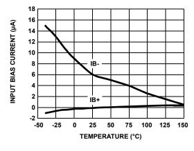
FIGURE 45. INPUT BIAS CURRENT vs TEMPERATURE
