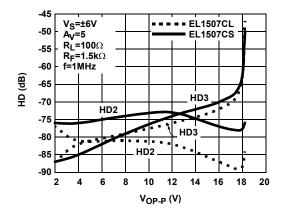
FIGURE 29. DIFFERENTIAL HARMONIC DISTORTION VS
