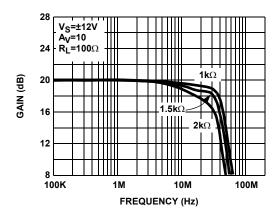
FIGURE 5. DIFFERENTIAL FREQUENCY RESPONSE vs R<sub>F</sub> (EL1507CS - 1/2 POWER MODE)
