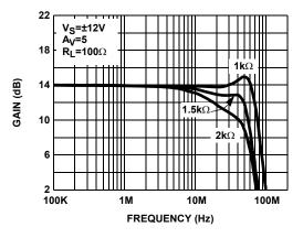
FIGURE 10. DIFFERENTIAL FREQUENCY RESPONSE vs R<sub>F</sub>
