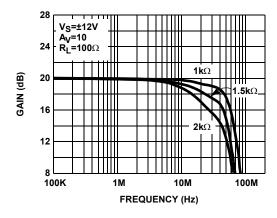
FIGURE 9. DIFFERENTIAL FREQUENCY RESPONSE vs R<sub>F</sub> (EL1507CL - 3/4 POWER MODE)
