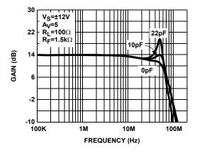
FIGURE 15. FREQUENCY RESPONSE vs C<sub>LOAD</sub> (EL1507CS - 3/4 POWER MODE)
