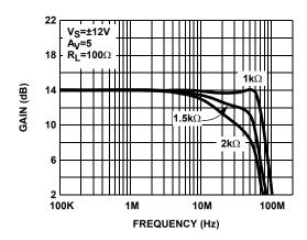
FIGURE 4. DIFFERENTIAL FREQUENCY RESPONSE vs R<sub>F</sub> (EL1507CS - 3/4 POWER MODE)
