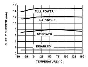
FIGURE 43. POSITIVE SUPPLY CURRENT vs TEMPERATURE
