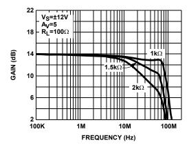
FIGURE 8. DIFFERENTIAL FREQUENCY RESPONSE vs R<sub>F</sub> (EL1507CL - FULL POWER MODE)
