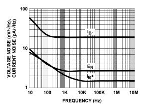
FIGURE 36. VOLTAGE AND CURRENT NOISE vs FREQUENCY
