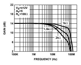
FIGURE 2. DIFFERENTIAL FREQUENCY RESPONSE vs  $R_F$  (EL1507CS - FULL POWER MODE)
