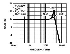
FIGURE 17. FREQUENCY RESPONSE vs C<sub>LOAD</sub> (EL1507CS - 1/2 POWER MODE)
