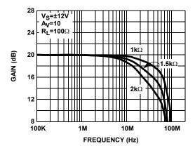
FIGURE 7. DIFFERENTIAL FREQUENCY RESPONSE vs R<sub>F</sub> (EL1507CL - FULL POWER MODE)
