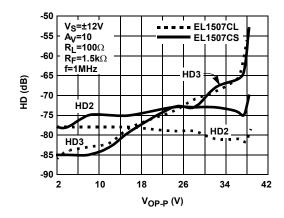
FIGURE 22. DIFFERENTIAL HARMONIC DISTORTION VS
