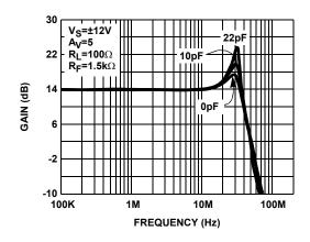
FIGURE 18. FREQUENCY RESPONSE vs C<sub>LOAD</sub> (EL1507CL - 1/2 POWER MODE)
