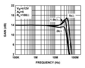
FIGURE 6. DIFFERENTIAL FREQUENCY RESPONSE vs R<sub>F</sub> (EL1507CS - 1/2 POWER MODE)
