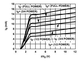
FIGURE 21. SUPPLY CURRENT vs SUPPLY VOLTAGE
