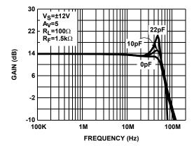
FIGURE 16. FREQUENCY RESPONSE vs C<sub>LOAD</sub> (EL1507CL - 3/4 POWER MODE)
