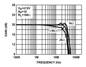
FIGURE 11. DIFFERENTIAL FREQUENCY RESPONSE vs R<sub>F</sub> (EL1507CL - 1/2 POWER MODE)
