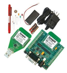
The EK2100 evaluation kit comes with management software, a power supply, an external battery holder, a pair of AA batteries, a screwdriver and a bag of components. (refer to the EK2100 Kit Contents document.) The kit also contains two different kinds of SNAP demonstration boards, each with a SNAP Engine:
