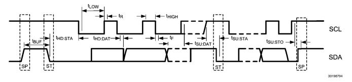
FIGURE 4. SMBus Timing Parameters
