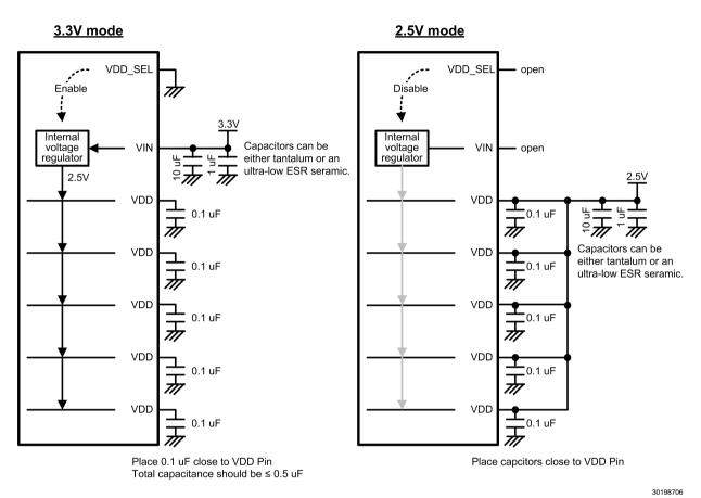
FIGURE 5. 3.3V or 2.5V Supply Connection Diagram
