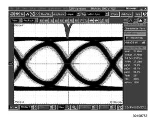
FIGURE 21. TL1 = 8-meter 30-AWG 100 Ohm Twin-axial Cable, 12 Gbps DS125BR401 settings: EQ[1:0] = R, 1 = 0F'h, DEM[1:0] = 0, 1
