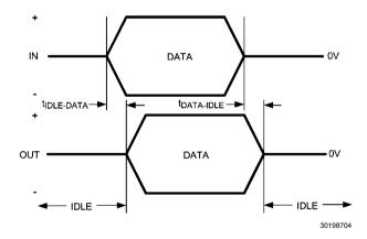
FIGURE 3. Transmit IDLE-DATA and DATA-IDLE Response Time
