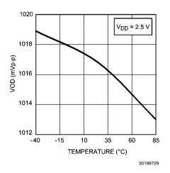
FIGURE 9. Output Differential Voltage (VOD = 1.0 Vp-p) vs. Temperature
