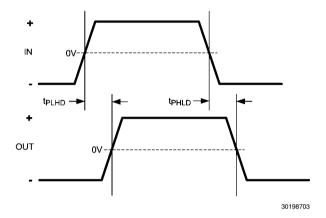
FIGURE 2. Propagation Delay Timing Diagram
