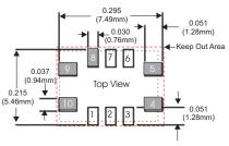
\* Do not route any traces in the keep out area. It is recommended the next layer under the keep out area is to be ground plane
