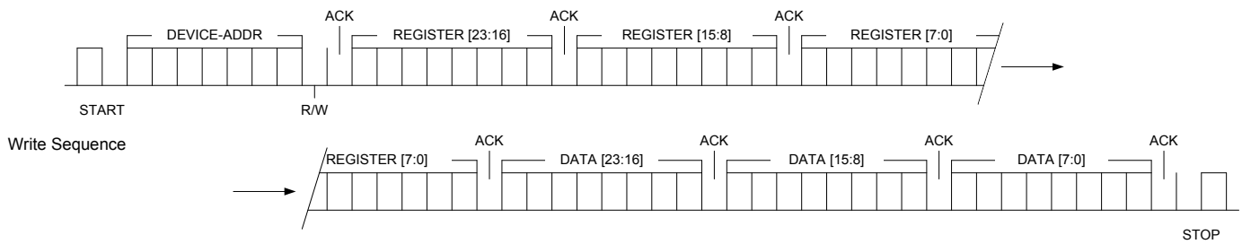
FIGURE 15. I 2 C WRITE SEQUENCE OPERATION
