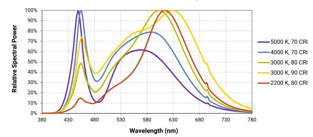
The following graph is the result of a series of pulsed measurements at 1100 mA and  $T_{J}$  = 85 °C.
