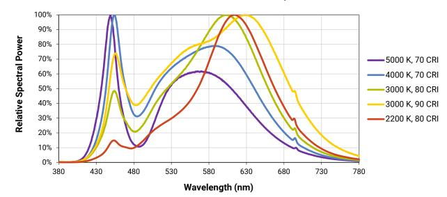
The following graphs are the result of a series of pulsed measurements at 500 mA and  $T_{J}$  = 85 °C.
