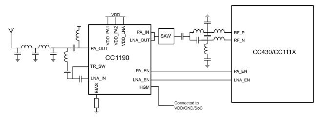
Figure 13. CC1190 + CC430/CC111X Application Circuit
