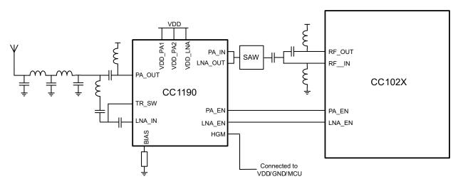
Figure 11. CC1190 + CC102X Application Circuit
