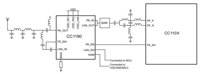
Figure 12. CC1190 + CC110X Application Circuit
