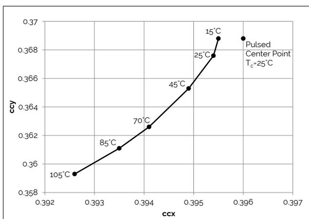
**Figure 15: 4000K Class A Color Shift vs. Case Temperature<sup>1</sup>**
