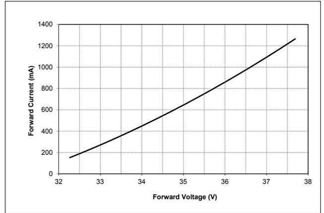
**Figure 3: Vero SE 13D Drive Current vs. Voltage**
