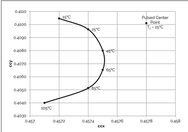
**Figure 11: 3000K, 97 CRI Color Shift vs. Case Temperature<sup>1</sup>**
