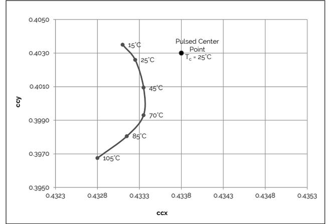
**Figure 12: 3000K, 90 CRI Color Shift vs. Case Temperature<sup>1,3</sup>**
