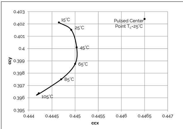
**Figure 13: 3000K Class A Color Shift vs. Case Temperature<sup>1</sup>**
