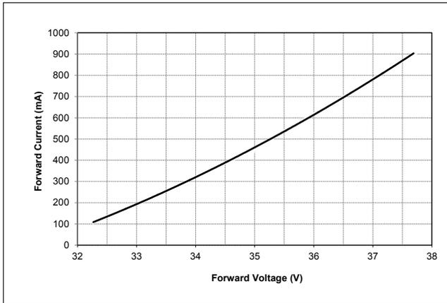
**Figure 2: Vero SE 13C Drive Current vs. Voltage**
