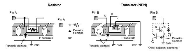
Fig.17 Example of monolithic IC structure
