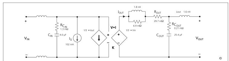
**Figure 22** — This model characterizes the AC operation of the bus converter including response to output load or input voltage transients or steady state modulations. The model enables estimates or simulations of input and output voltages under transient conditions, including response to a stepped load with or without external filtering elements.
