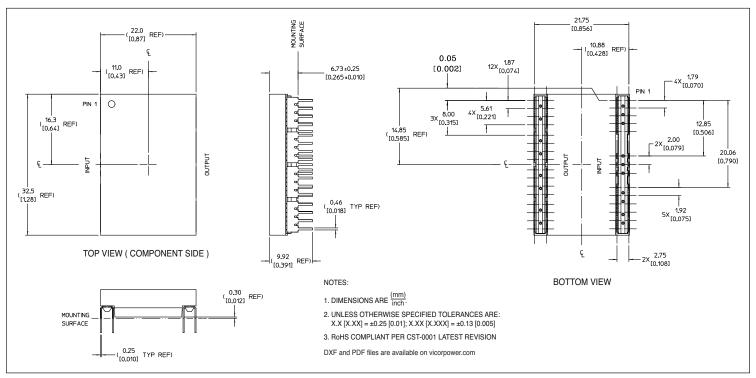
Figure 17 — BCM<sup>®</sup> through-hole module mechanical outline
