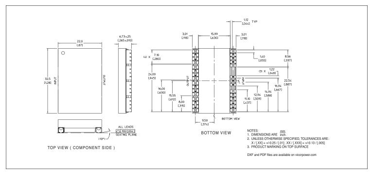
Figure 15 — BCM<sup>®</sup> module J-Lead mechanical outline; onboard mounting
