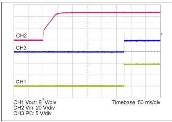
Figure 3 — Output voltage turn on waveform with input turn on at full load and 48  $V_{\rm IN}$
