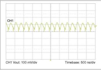
$\begin{array}{l} \textit{Figure 7} & - & \textit{Output voltage ripple at full load and 48 } V_{\textit{IN}} \\ & \textit{without any external bypass capacitor.} \end{array}$
