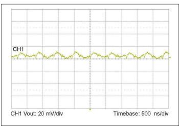
**Figure 8** — Output voltage ripple at full load and 48 V<sub>IN</sub> with 10 μF ceramic external bypass capacitor and 20 nH of distribution inductance.
