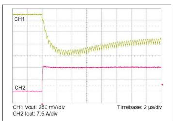
**Figure 10** — 0 – 15 A load step with 100 µF input capacitor and no output capacitor.
