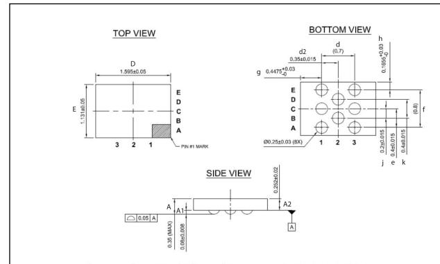
NOTE: BACKSIDE LAMINATE IS INCLUDED IN THE OVERALL DIE THICKNESS DIMENSION.
