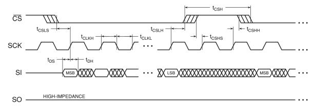
Figure 15-2. Serial Output Timing
