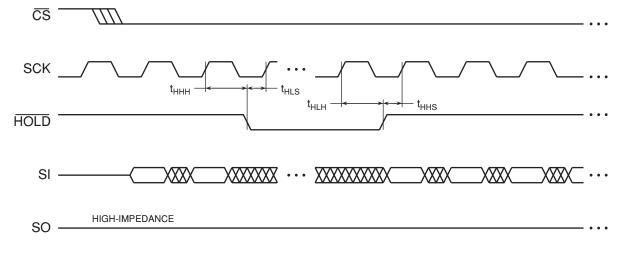
Figure 15-5. HOLD Timing – Serial Output
