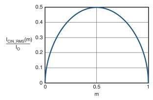
Figure 2. I<sub>CIN</sub> vs. Voltage Conversion Ratio
