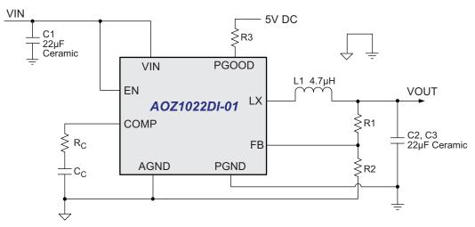
Figure 1. 3.3V/3A Synchronous Buck Regulator
