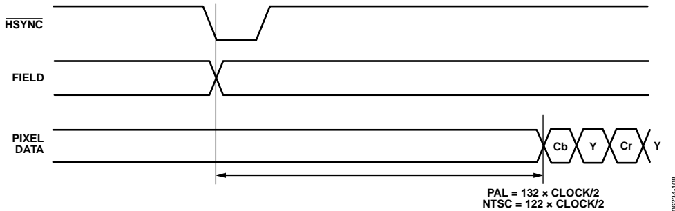
Figure 110. SD Timing Mode 1, Odd/Even Field Transitions (Master/Slave)
