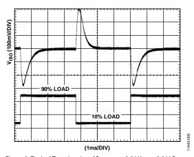
Figure 9. Typical Transient Load Response, 3.3 V Input 3.3 V Output, 10% to 90% Load Step
