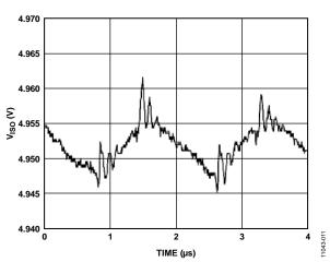
Figure 11. Typical V<sub>ISO</sub> = 5 V Output Voltage Ripple at 90% Load
