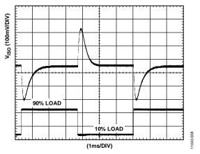
Figure 8. Typical V<sub>ISO</sub> Transient Load Response, 5 V Input, 5 V Output, 10% to 90% Load Step
