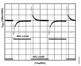
Figure 10. Typical Transient Load Response, 5 V Input, 3.3 V Output, 10% to 90% Load Step
