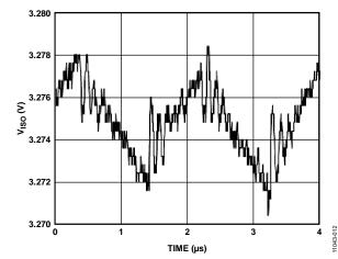
Figure 12. Typical V<sub>ISO</sub> = 3.3 V Output Voltage Ripple at 90% Load
