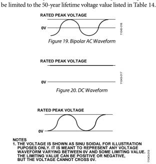
Figure 21. Unipolar AC Waveform
