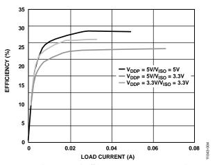
Figure 4. Typical Power Supply Efficiency at 5 V/5 V, 5 V/3.3 V, and 3.3 V/3.3 V
