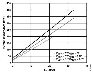
Figure 5. Typical Total Power Dissipation vs. I<sub>ISO</sub>
