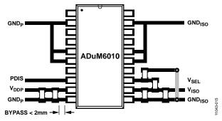
Figure 18. Recommended PCB Layout
