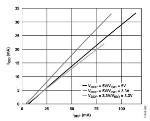
Figure 6. Typical Isolated Output Supply Current, I $_{\rm ISO}$ , as a Function of External Load, at 5 V/5 V, 5 V/3.3 V, and 3.3 V/3.3 V
