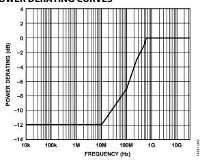
Figure 2. Power Derating for Through Path vs. Frequency, T<sub>CASE</sub> = 85°C
