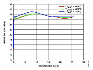
Figure 12. Input 0.1 dB Power Compression (P0.1dB) vs. Frequency over Temperature
