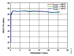
Figure 14. Input IP3 vs. Frequency over Temperature
