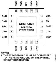
Figure 5. Pin Configuration (Top View)
