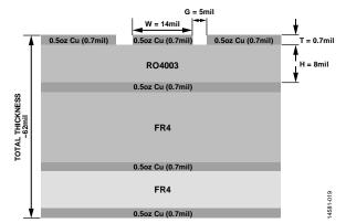
Figure 19. Evaluation Board (Cross Sectional View)
