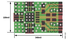
Figure 22. Probe Board Layout (Top View)
