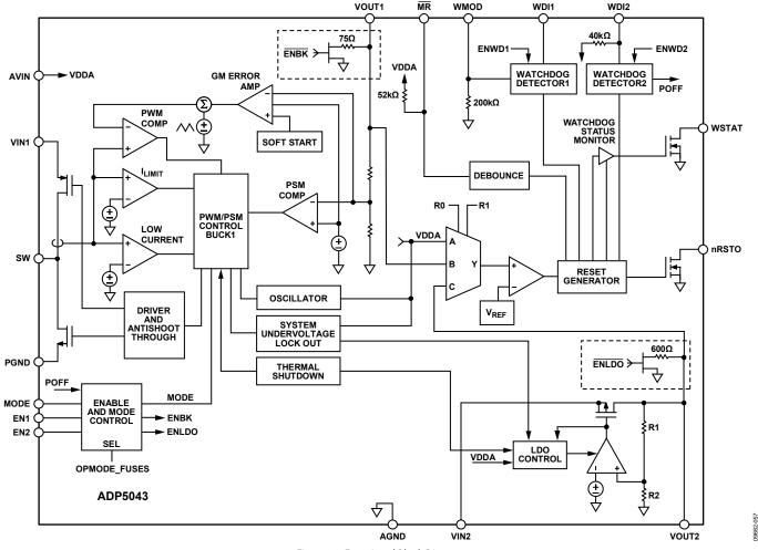
Figure 43. Functional Block Diagram
