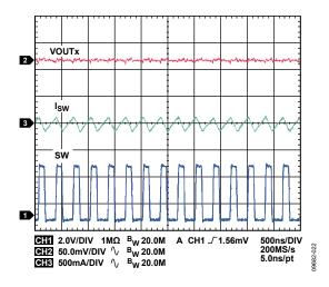
Figure 21. Typical Waveforms, VOUT1 = 1.8 V, IOUT1 = 30 mA, PWM Mode
