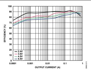
Figure 12. Buck Efficiency vs. Load Current, Across Input Voltage,  $V_{OUT1} = 1.8$  V, Auto Mode
