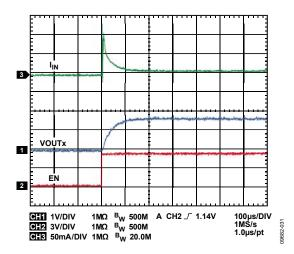
Figure 29. LDO Startup, VOUT2 = 3.3 V, IOUT2 = 5 mA
