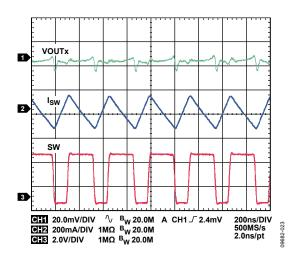
Figure 22. Typical Waveforms, VOUT1 = 3.3 V, IOUT1 = 30 mA, PWM Mode
