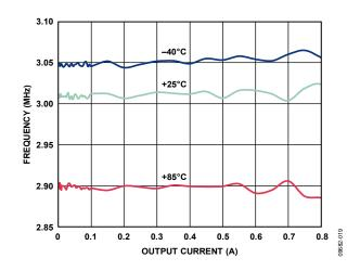
Figure 18. Buck Switching Frequency vs. Output Current, Across Temperature, V<sub>OUT1</sub> = 1.8 V, PWM Mode
