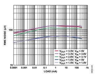
Figure 38. LDO Output Noise vs. Load Current, Across Input and Output Voltage
