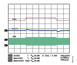
Figure 23. Buck Response to Line Transient, Input Voltage from 4.5 V to 5.0 V,  $V_{OUTI} = 3.3$  V, PWM Mode
