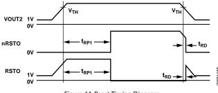
Figure 44. Reset Timing Diagram
