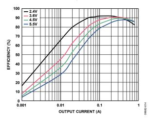
Figure 13. Buck Efficiency vs. Load Current, Across Input Voltage,  $V_{OUTI}$  = 1.8 V, PWM Mode
