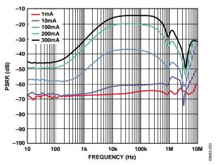
Figure 41. LDO PSRR vs. Frequency, VIN2 = 3.1 V, VOUT2 = 2.8 V
