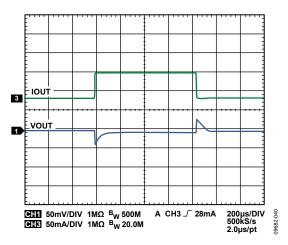
Figure 35. LDO Response to Load Transient,  $I_{OUT2}$  from 1 mA to 80 mA,  $V_{OUT2} = 3.3 V$
