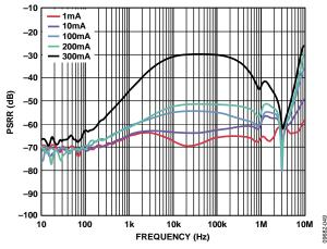
Figure 40. LDO PSRR Across Output Load,  $V_{IN2} = 3.3 V$ ,  $V_{OUT2} = 2.8 V$
