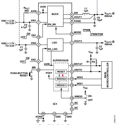
Figure 56. Application Diagram
