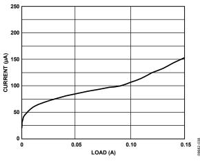
Figure 33. LDO Ground Current vs. Output Load, Vout2 = 2.8 V
