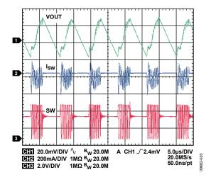
Figure 19. Typical Waveforms, Vouti = 3.3 V, Iouti = 30 mA, Auto Mode
