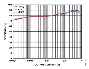
Figure 16. Buck Efficiency vs. Load Current, Across Temperature,  $V_{OUT1} = 1.8 V$ , Auto Mode
