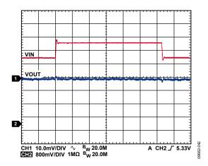
Figure 36. LDO Response to Line Transient,  $V_{IN2} = 4.5 V$  to 5.5 V,  $V_{OUT2} = 3.3 V$
