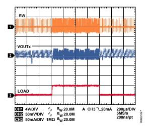
Figure 26. Buck Response to Load Transient,  $I_{OUT2}$  from 1 mA to 50 mA,  $V_{OUT1} = 1.8$  V, Auto Mode
