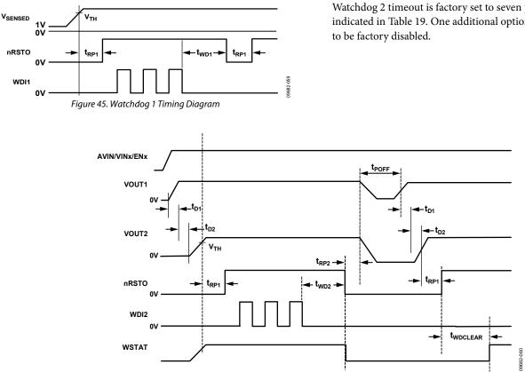
Figure 46. Watchdog 2 Timing Diagram (Assuming that VOUT2 is the Monitored Rail)
