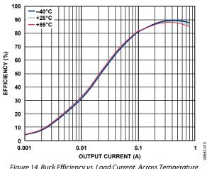
Figure 14. Buck Efficiency vs. Load Current, Across Temperature,  $V_{OUT1} = 1.8 V$ , PWM Mode
