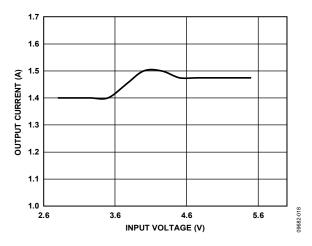
Figure 17. Buck DC Current Capability vs. Input Voltage, Vouti = 1.8 V
