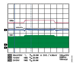
Figure 24. Buck Response to Line Transient,  $V_{IN} = 4.5$  V to 5.0 V,  $V_{OUTI} = 1.8$  V, PWM Mode
