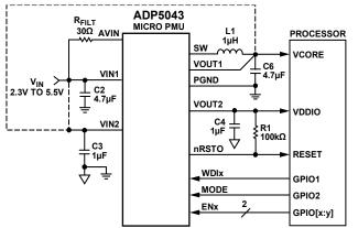
Figure 50. Processor System Power Management with PSM/PWM Control
