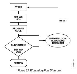
The second watchdog, refreshed through the WDI2 pin, is useful in applications where safety is a very critical factor and the system must recover from unexpected operations, for example, a processor stuck in a continuous loop where Watchdog 1 is kept refreshed or environmental conditions that may unset or damage the processor port controlling the WDI1 pin. In the event of a Watchdog 2 timeout, the ADP5043 power cycles all the supplied rails to guarantee a clean processor start.
