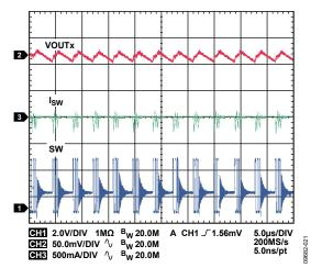
Figure 20. Typical Waveforms, Vout1 = 1.8 V, Iout1 = 30 mA, Auto Mode
