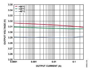
Figure 31. LDO Load Regulation Across Temperature,  $V_{\text{IN2}}$  = 3.6 V,  $V_{\text{OUT2}}$  = 3.3 V
