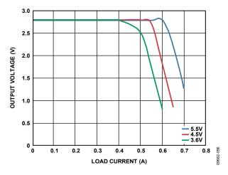
Figure 37. LDO Output Current Capability vs. Output Voltage
