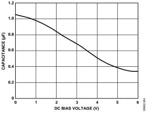
Figure 51. Capacitance vs. Voltage Characteristic
