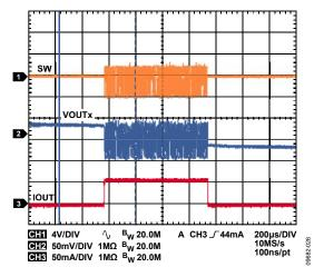
Figure 25. Buck Response to Load Transient,  $I_{OUT1}$  from 1 mA to 50 mA,  $V_{OUT1} = 3.3 V$ , Auto Mode
