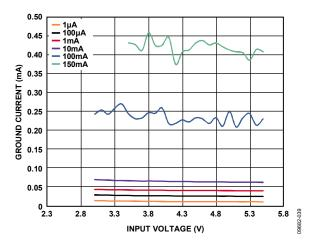
Figure 34. LDO Ground Current vs. Input Voltage, Across Output Load,  $V_{OUT2} = 2.8 V$
