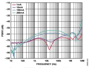
Figure 42. LDO PSRR vs. Frequency,  $V_{IN2} = 5 V$ ,  $V_{OUT2} = 3.3 V$
