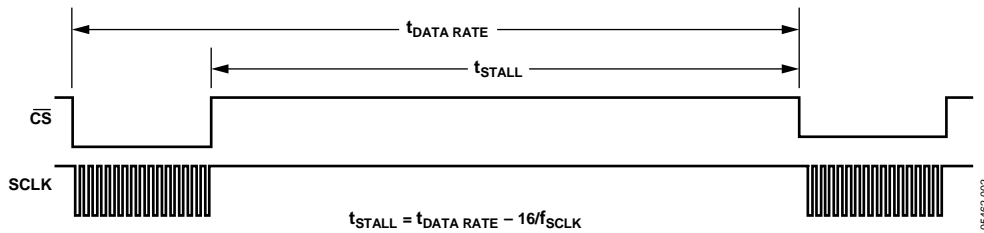
Figure 2. SPI Chip Select Timing
