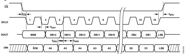
Figure 2. SPI Timing and Sequence
