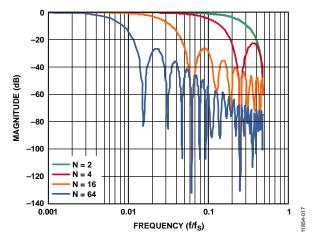
Figure 17. Bartlett Window FIR Filter Frequency Response
