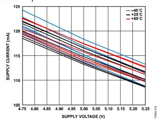
Figure 21. Supply Current vs. Supply Voltage
