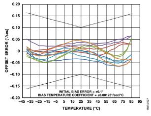
Figure 9. Offset (Bias) Error vs. Temperature,  $-40^{\circ}$ C to  $+85^{\circ}$ C to  $-40^{\circ}$ C
