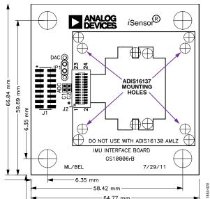
Figure 22. Physical Diagram for the ADIS16IMU1/PCBZ
