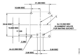
Figure 24. Suggested Mounting Hole Locations, Connector Down
