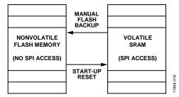
Figure 16. SRAM and Flash Memory Diagram
