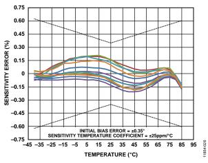
Figure 8. Sensitivity Error vs. Temperature,  $-40^{\circ}$ C to  $+85^{\circ}$ C to  $-40^{\circ}$ C
