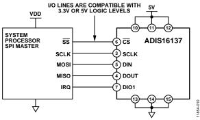
Figure 10. Electrical Connection Diagram
