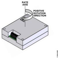
Figure 6. Axial Orientation (Bottom Side Facing Up)
