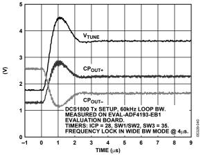
Figure 10. V<sub>TUNE</sub> Settling Transient for a 75 MHz Jump from 1818 MHz to 1893 MHz with Sirenza 1843T VCO
