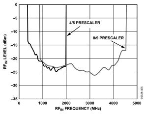
Figure 7. RF Input Sensitivity
