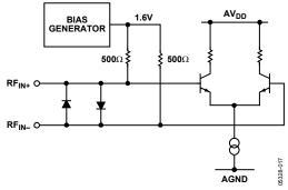
Figure 21. RF Input Stage
