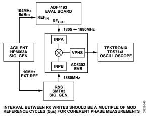
Figure 19. Test Setup for Phase Lock Time Measurement
