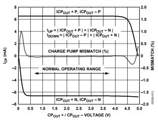
Figure 12. Differential Charge Pump Output Compliance Range and Charge Pump Mismatch with  $V_P1 = V_P2 = 5 V$
