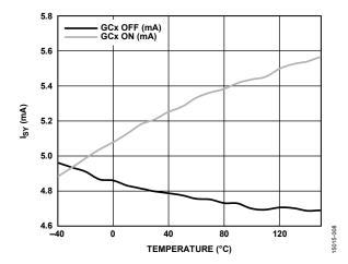
Figure 8. Supply Current (Isy) Per Channel vs. Temperature,  $V_{DD} = 5 V$
