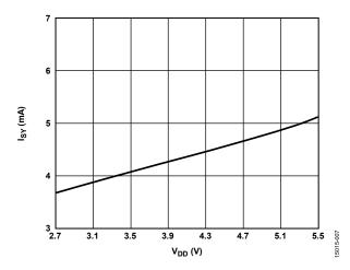
Figure 7. Supply Current ( $I_{SY}$ ) Per Channel vs. Supply Voltage ( $V_{DD}$ ),  $T_A = 25^{\circ}$ C
