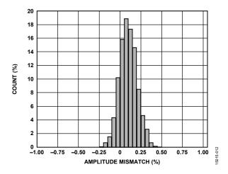
Figure 12. VSINx to VCOSx Amplitude Mismatch Per Channel
