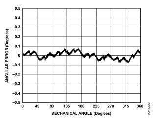
Figure 4. Error Waveform After Offset and Amplitude Correction, Assuming Homogeneous Aligned Magnetic Field Over One Channel
