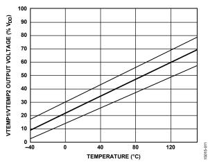
Figure 11. VTEMP1/VTEMP2 Output Voltage vs. Temperature
