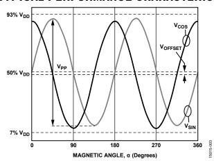
Figure 3. Raw Output Waveforms
