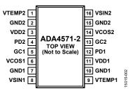
Figure 2. Pin Configuration
