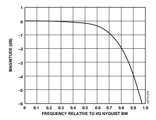
Figure 16. Cascaded Filter Pass-Band Detail (N = 3)
