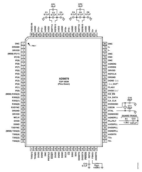
Figure 4. Basic Connection Diagram
