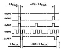
Figure 7. Σ-Δ Output Signals
