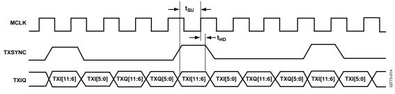
Figure 14. Transmit Path Timing
