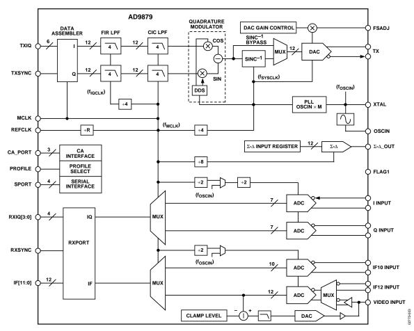
Figure 3. Block Diagram
