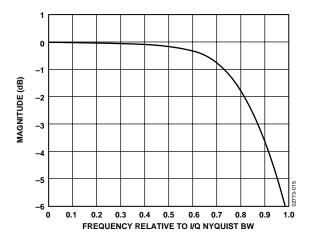
Figure 15. Cascaded Filter Pass-Band Detail (N = 4)
