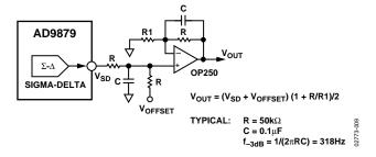
Figure 9.  $\Sigma$ - $\Delta$  Active Filter with Gain and Offset
