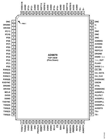
Figure 2. Pin Configuration
