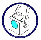
2. Do not directly touch or handle the silicone lens surface. It may damage the internal circuitry.
