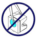
3. As silicone encapsulation is permeable to gases, some corrosive substances such as  $H_2S$  might corrode silver plating of leadframe. Special care should be taken if an LED with silicone encapsulation is to be used near such substances.
