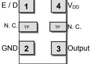
Terminations as viewed from the Top NOTE: XPRESSO HCMOS XOs are designed to fit on Industry Standard, 4 pad layouts
