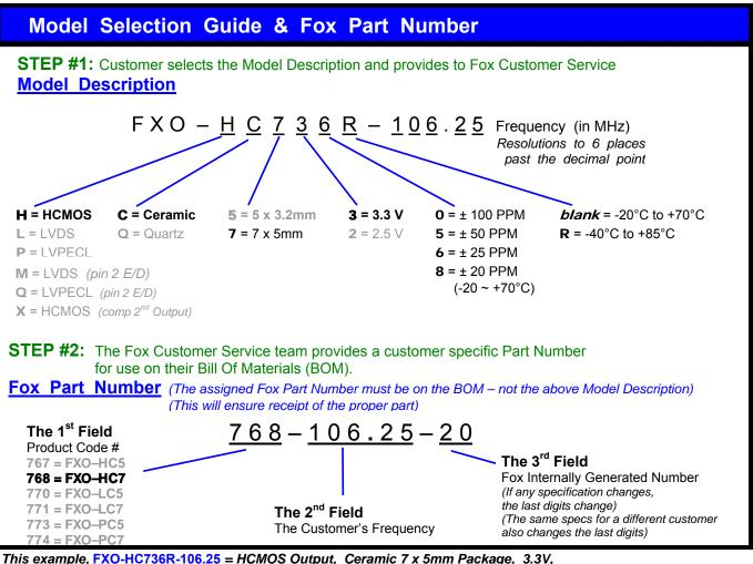
.25 = HCMOS Output, Ceramic 7 x 5mm Package, 3.3V, ±25 PPM Stability, -40 to +85°C Temperature Range, at 106.25 MHz
