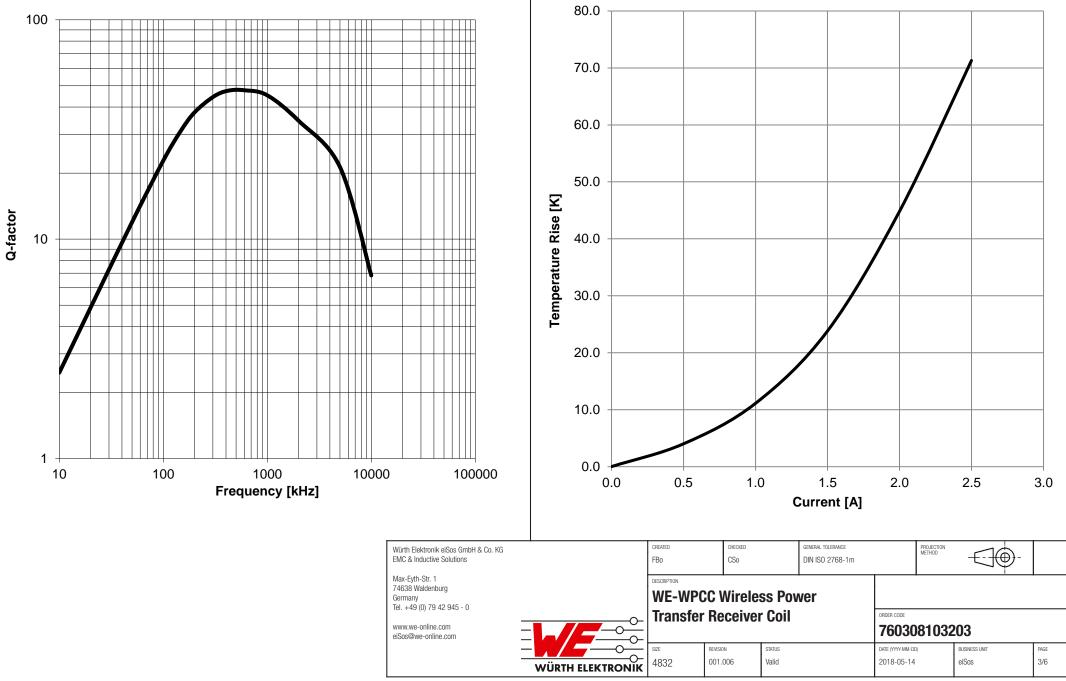
**Typical Temperature Rise vs. Current Characteristics:**
