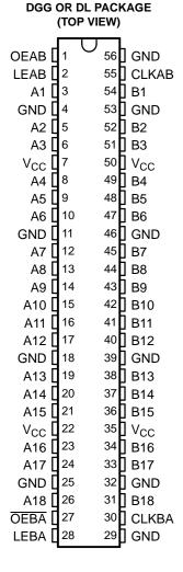
Data flow for B to A is similar to that of A to B, but uses  $\overline{\text{OEBA}}$ , LEBA, and CLKBA. The output enables are complementary (OEAB is active high, and  $\overline{\text{OEBA}}$  is active low).
