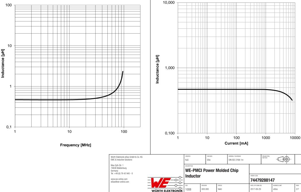
**Typical Inductance vs. Frequency Characteristics:**
