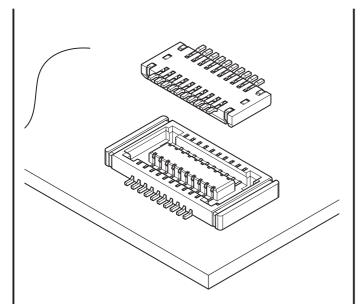
This JAN connector is a board-to-board connector with stacking height 1.0 mm and 0.4 mm pitch, which is the lowest-profile connector in the [electro mechanical component] industry.
