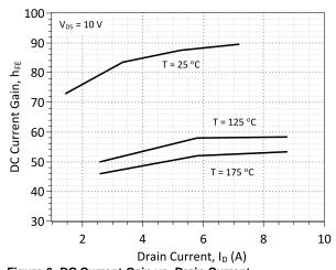
Figure 6: DC Current Gain vs. Drain Current
