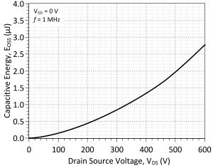
Figure 10: Output Capacitance Stored Energy
