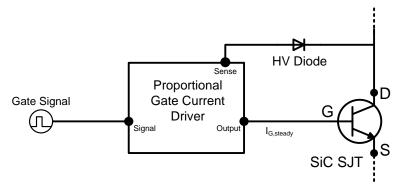
Figure 18: Simplified Voltage Controlled Proportional Driver
