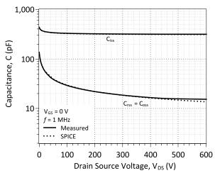
Figure 9: Input, Output, and Reverse Transfer Capacitance
