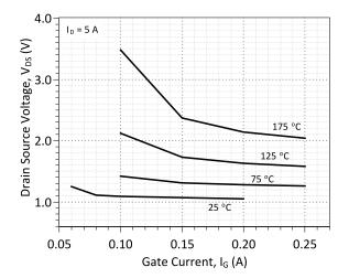
Figure 4: Drain-Source Voltage vs. Gate Current
