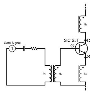
Figure 19: Simplified Current Controlled Proportional Driver
