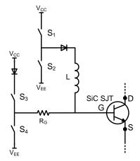
Figure 17: High Speed, Low-Loss Driver with Boost Inductor Topology
