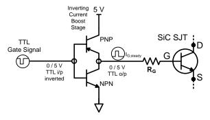
Figure 15: Simple TTL Gate Drive Topology
