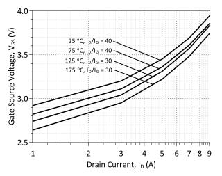
Figure 7: Typical Gate - Source Saturation Voltage
